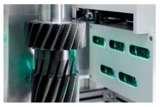
Optional tactile probing system for lengths and axial run-out
