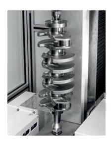
Opticline CA618-AE for measuring crank shafts
