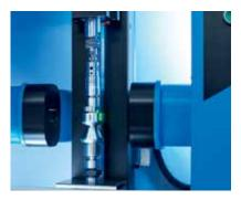
Simple clamping of the workpiece between tips
