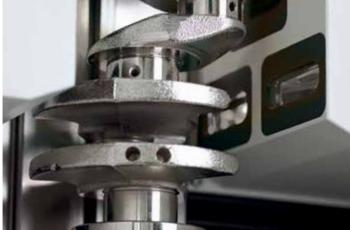
Optional tactile probing system for concentric lengths and axial run-outs
