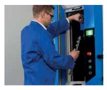
Simple operation of the measuring machine thanks to fast tailstock adjustment
