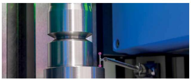
Optional tactile probing system for additional form measurements
