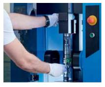
Workpieces weighing up to 15 kg can be measured with the Opticline CS series
