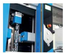
Integrated light barrier to protect operators in accordance with international safety standards
