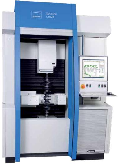
Opticline C1023 with safety light barrier and roller shutter
